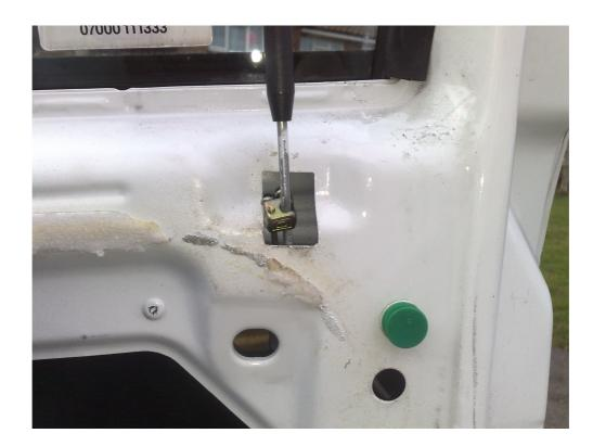
Here is the picture of the motor inside the door, you can see which way the motor faces and see that it will not interfere with the window as it is behind the window guide.
