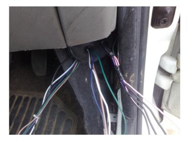
5. Remove the rubber channel from outside (use a flat head screwdriver as leverage). Push the cables outside and put them through the rubber channel you just removed. Put the rubber channel back on (use a screwdriver to push this back in).
