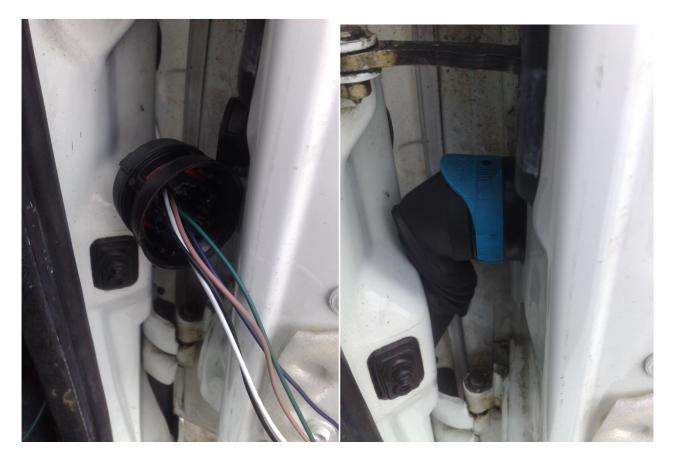
7. Now your wires are through to the door you should now fit the motors to the door. To do this remove the nut circled below, this is the window guide. On the picture below you see the metal strip which I have used to screw onto, the bottom hole is already there but the top hole needs to be drilled out.
