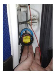
Now I cut these cables off the connector as I only had 4 speaker cables going through this. If you have electric windows I would suspect that these cables will go through this connector too, so I wouldn't follow this next bit.
