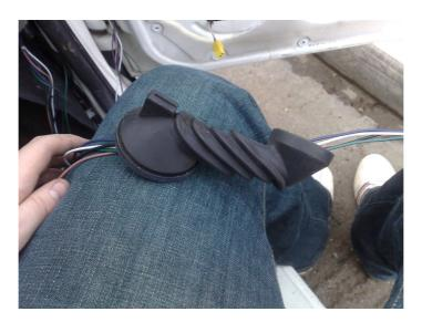
6. Put the cut plastic connectors back on and thread the cables through them. Connect it all back up and put the blue clip down, you now have the wires through to the door and kept it waterproof.
